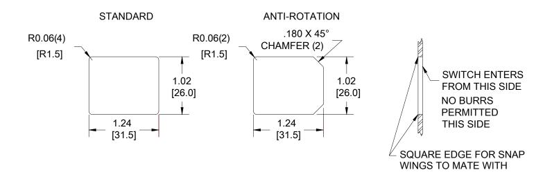
Designed for panel thicknesses up to .060, .085, and .105, including paint and other coverings applied to panel.
