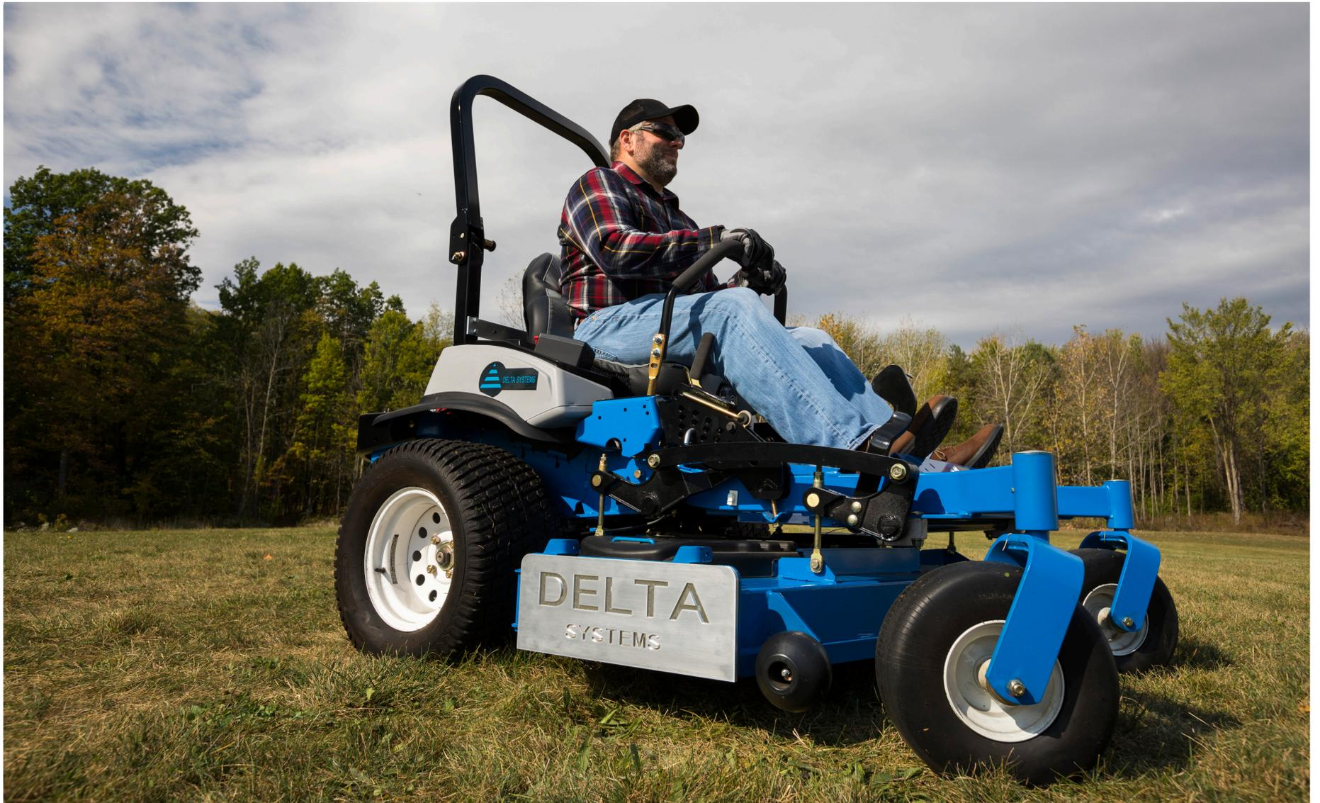
To demonstrate its range of control and connectivity solutions, Ohio-based Delta Systems developed a pair of Tech Tractors, including one based on an Exmark commercial zero-turn radius mower. The Tech Tractor incorporates a range of technologies, including a pushbutton start system, touchscreen display, backup camera and object detection system and Bluetooth-enabled monitoring system.
