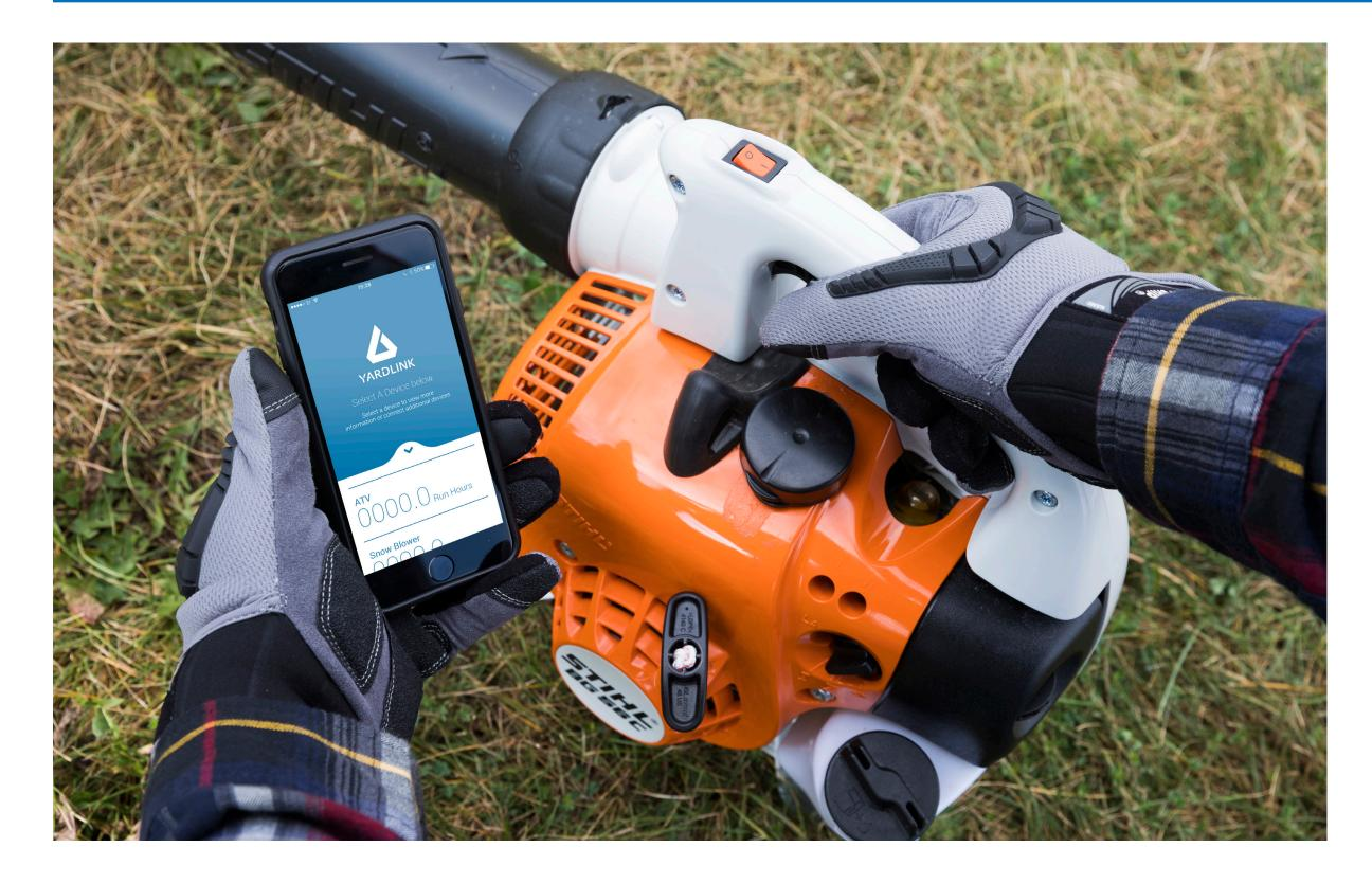
Delta Systems YardLink is a Bluetooth-enabled, puck-like portable device that can be mounted to any type of engine-powered equipment. Working through the Delta Blue app, YardLink uses engine vibration to track parameters such as engine hours and battery status. Multiple YardLink units can be read through the app, providing the ability to monitor fleets of machines.
